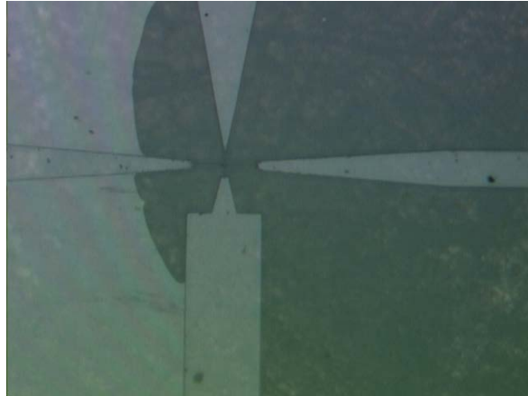
Figure 4.12 This micrograph shows the Loctite 3301 UV curable adhesive flowing through the micro channel. Drops of Loctite were applied to the cover slip edge to the middle right outside of the viewable picture. The adhesive is flowing from right to left. A pool of adhesive is shown collecting on the left side of the microchannel. The adhesive flowed through the microchannel (destroying it) from the right to the left.
