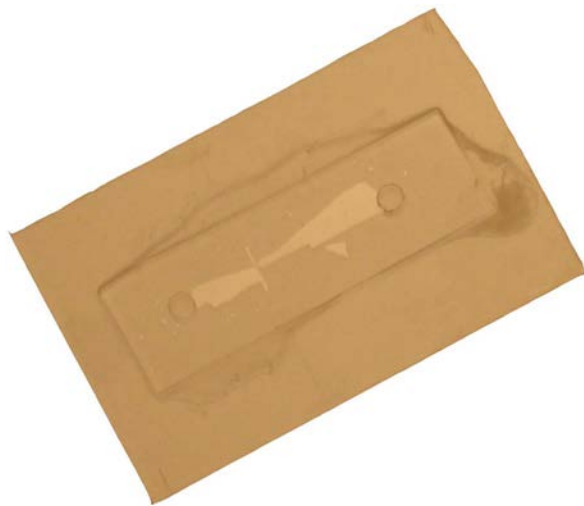
Figure 4.13 This figure shows a test sample half slide patterned with the microchannel device pattern in SU-8 and with a cover slip that is the full 30 millimeters in length. It has through holes drilled through at the original design dimensions of 22 millimeters apart. Large droplets of adhesive were used. The channel was destroyed when adhesive flowed into the channel.
