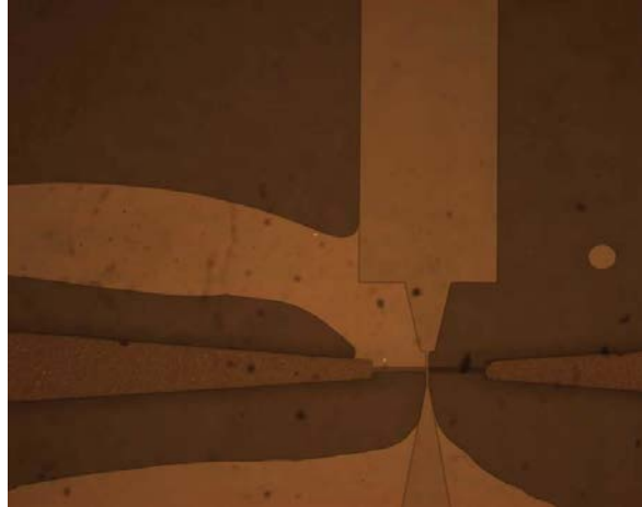
Figure 4.14 This figure shows device MC-06 during cover slip bonding. A large air bubble is shown in the upper right adjacent to the microchannel. The bottom of the picture shows the boarder between adhesive and unbonded SU-8 and glass. The adhesion process failed while attempting to fill the lower regions shown in this picture with epoxy.
